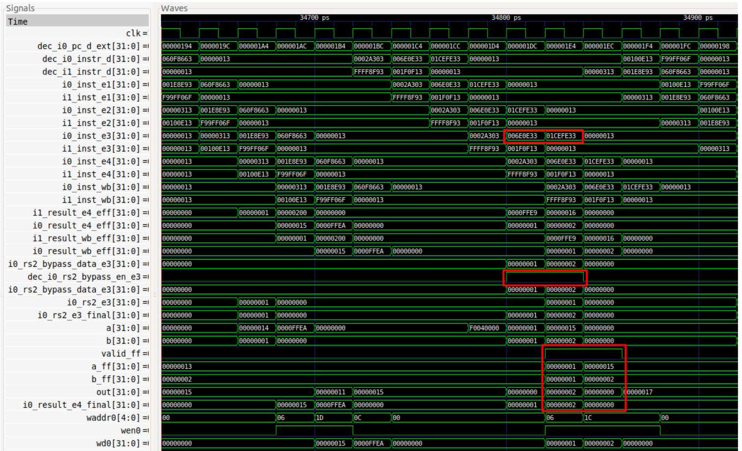
Both the dependent add and and instructions use the secondary ALU for recalculating the result. Note that the second input operand for the and instruction is bypassed at EX3.
