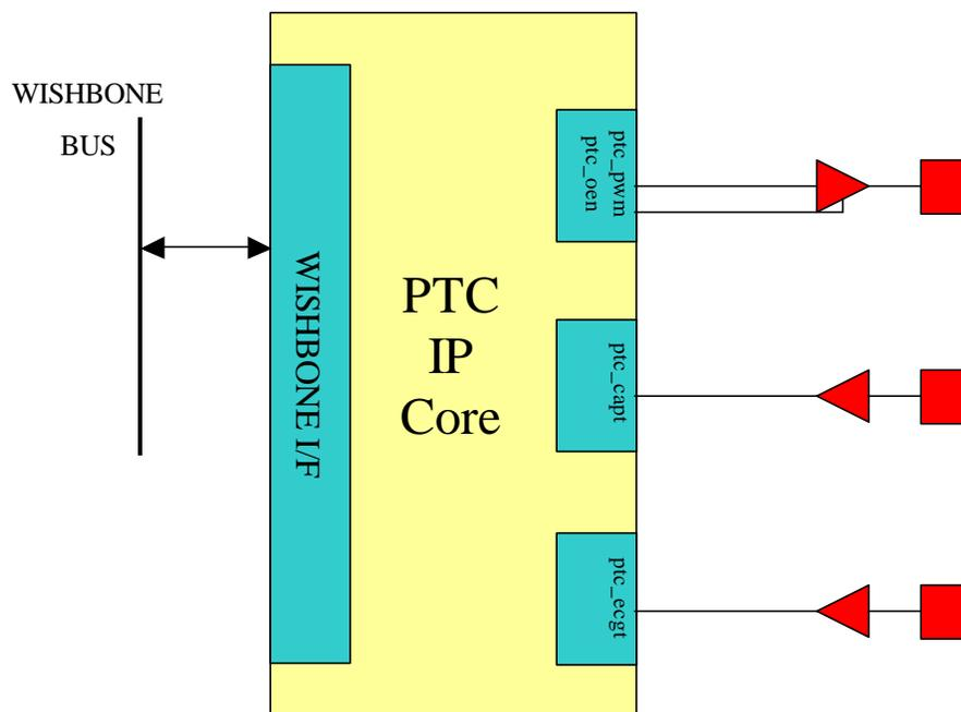
Figure 3. Core's Interfaces
