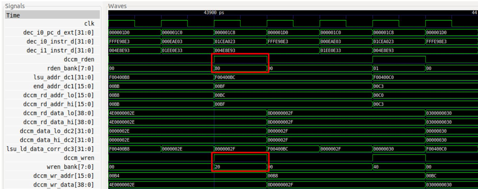
In this case, the DCCM read and DCCM write occur in the same cycle. However, because they are to different banks, they can be performed in the same cycle.
