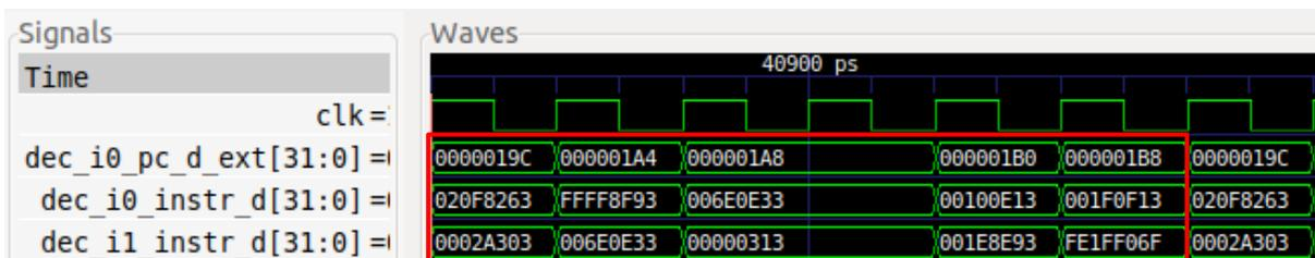
After the `lw` (0x0002a303), the dependent `add` instruction (0x006e0e33) is stalled for some cycles. 1 iteration takes 6 cycles.
