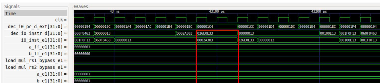
The second operand is bypassed from the value read by the load. This way, only 1 cycle is lost due to the dependency.
