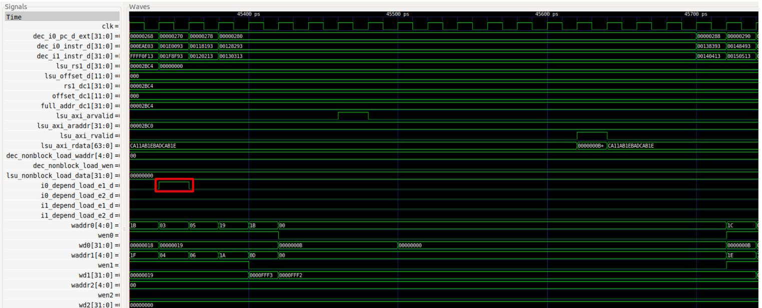
The RAW hazard is detected, the pipeline is stalled and the forwarding takes place as explained in the lab.
