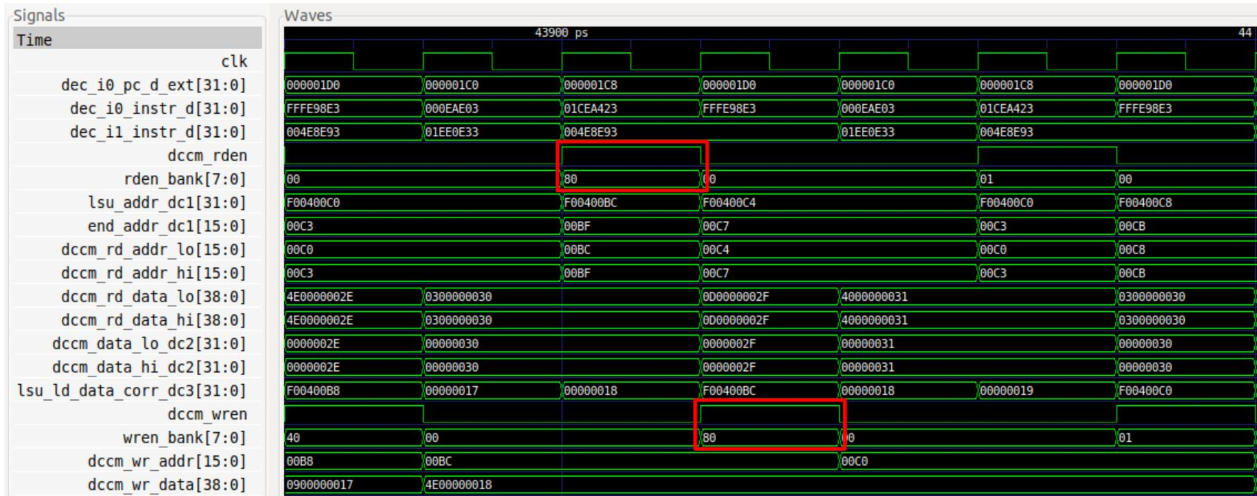
Again, the DCCM read and DCCM write occur in the same cycle. However, in contrast to the last example, the read and write are to the same bank, so the write is delayed one cycle.
