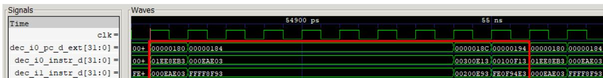
Like before, the dependent lw instruction must stall for 1 cycle, since one of its input operands is not available until the first add executes in EX1 and forwards the result.
