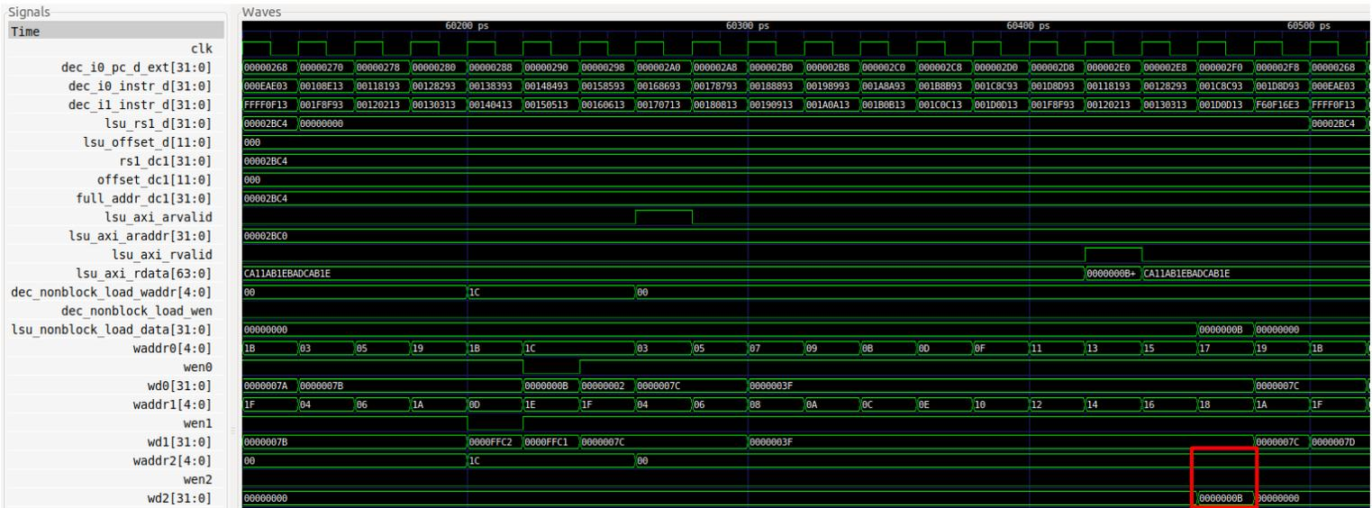
6) In the program Section 2.C of Lab 14 (available at [\[RVfpgaPath\]/RVfpga/Labs/Lab14/LW\\_Instruction\\_ExtMemory](#)), replace instruction `add x1, x1, 1` with `add x1, x28, 1`. This introduces a RAW hazard between the modified `add` instruction and the non-blocking load at the beginning of the loop (`lw x28, (x29)`). Analyse in simulation how this hazard is handled in SweRV EH1.
