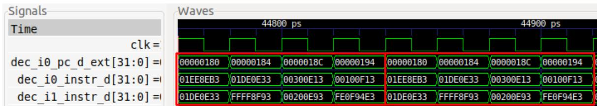
Now each iteration takes 4 cycles to execute as the dependent add instruction must stall for 1 cycle, since one of its input operands is not available until the first add executes in EX1 and forwards the result.
