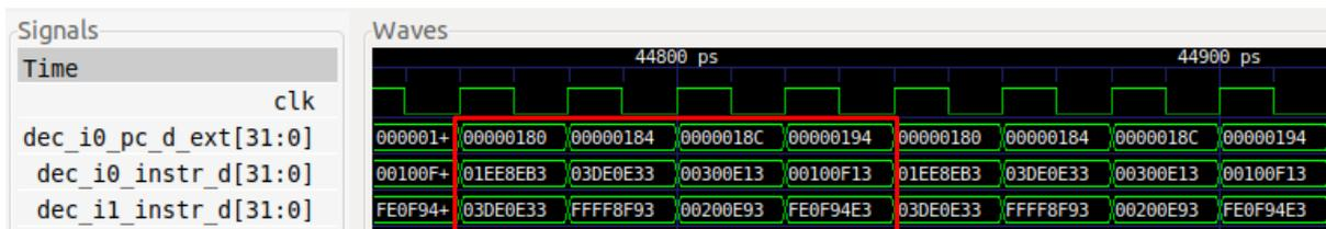
Like before, the dependent mul instruction must stall for 1 cycle, since one of its input operands is not available until the first add executes in EX1 and forwards the result.
