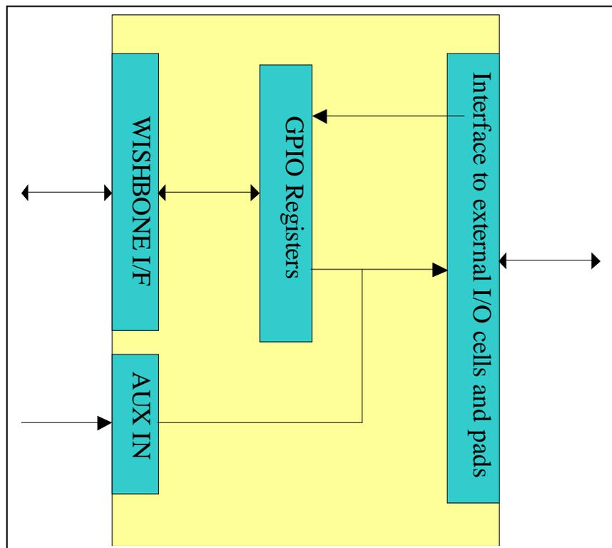
Figure 1. Core Architecture
